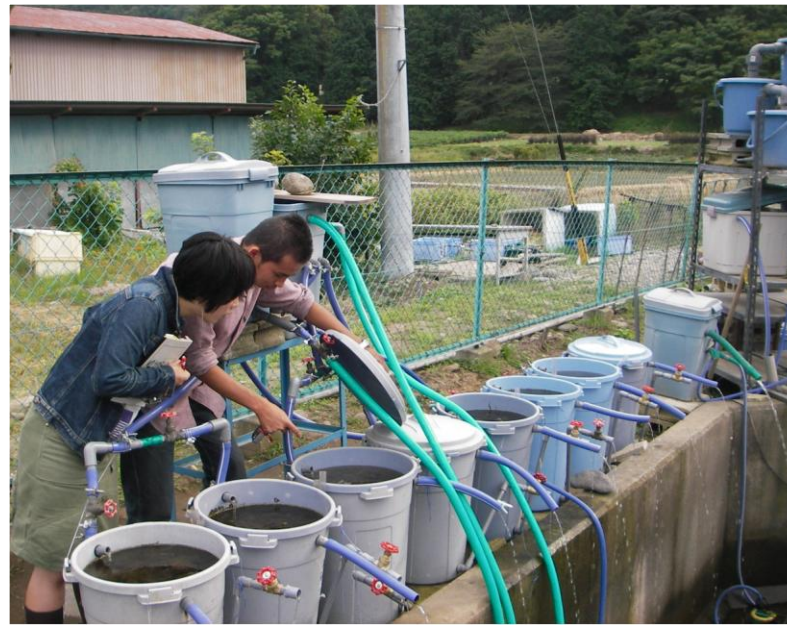
Filter resistance (NHL) of Open filter was almost constant. But the resistance of Covered filter increased almost every day.
