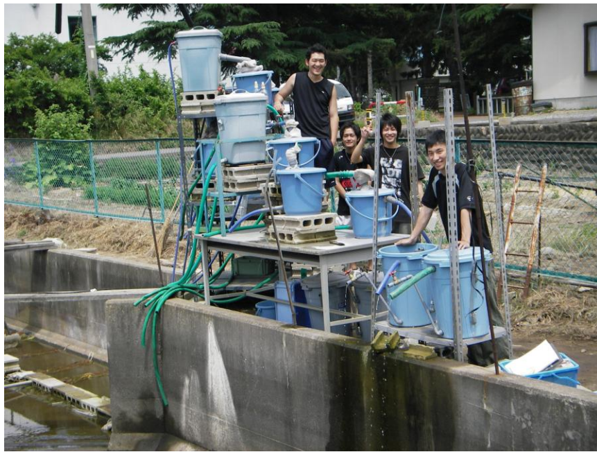
Multiple Roughing Filters to eliminate SS from an irrigation canal water.
