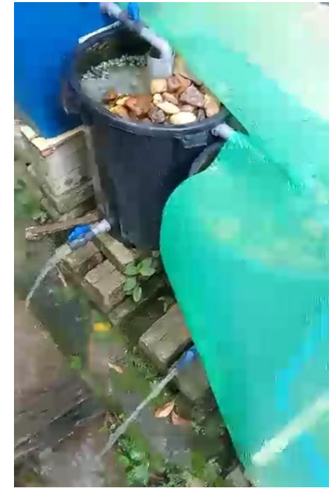
Backwashing up-flow roughing filter ⑧-163
