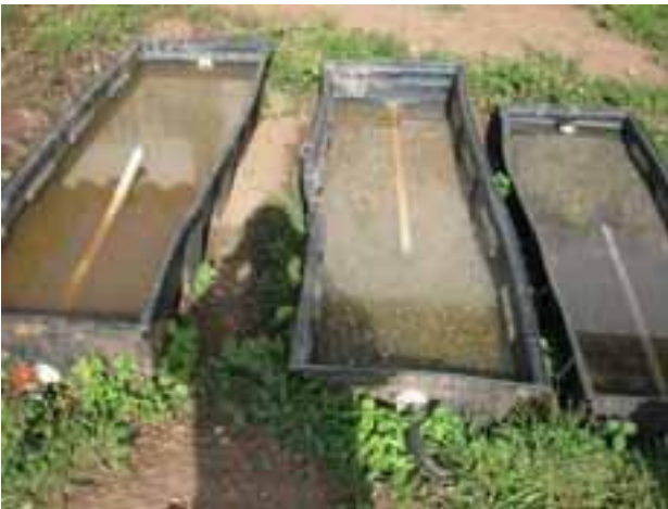
3 steps of gravel filters
