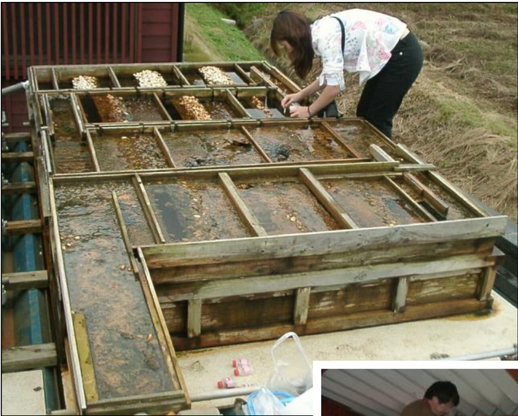
Final treatment of slow sand filter is in his garage.
