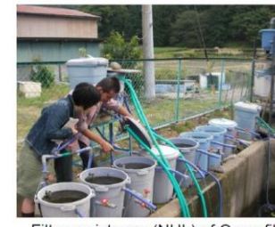
Filter resistance (NHL) of Open filter was almost constant. But the resistance of Covered filter increased almost every day.
