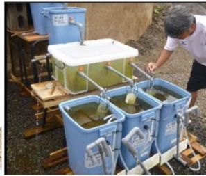
Different flow rate of sand filters (5m/d, 10m/d, 20m/d) All good quality of filtrates.
