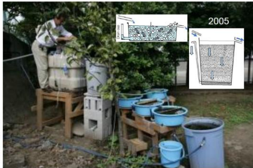
There are sedimentation tank, 4 gravel filters, and slow sand filter. Polluted water turns to safe and reliable water quality.
