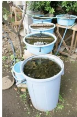
No detection of coli-form bacteria, lead, herbicides of Atrazine and Simazine. Nitrate N concentration : 2.0 mg/L, Nitrite N: 0 mg/L, pH8.5, total hardness: 250 mg/L and residual chlorine 0 mg/L.
