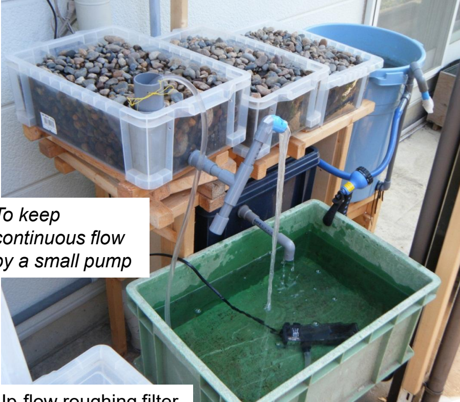
Up-flow roughing filter To make subsurface suspension free clean water in the flood plain.
