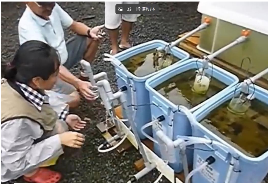
Small scale experiment model of Ecological Purification System to make safe and delicious drinking water was moved to Dave Parker Eco-Lodge, Apia, Samoa. February, 2013.
